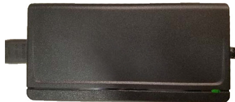
Power Supply LED lit
