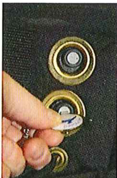
Remove fuse by inserting any side of keychain into slot. Push in and turn counterclockwise.
