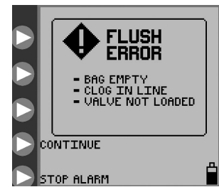
Figure 28. Flush Error screen.
