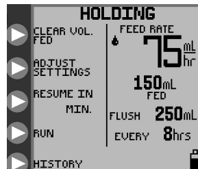
Figure 18A. HOLDING mode options, continuous feeding mode.
