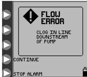
Figure 29. Flow Error screen.
