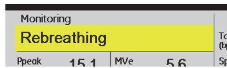
If several alarm conditions have been reached, the alarm descriptions are rolling in the display. A “>>” symbol is indicating that more than one alarm is set.
