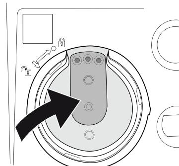
**1** Connect the insert to the ventilator. While connecting, the lock indicator on the insert's lock-ring should point to the unlock symbol on the Vivo 65.
