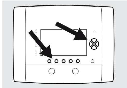
The navigation buttons are used to view the different sections indicated above each one. The same navigation button can also be used to view additional information in some sections, or it can be designated a temporary function while an event window is active.
