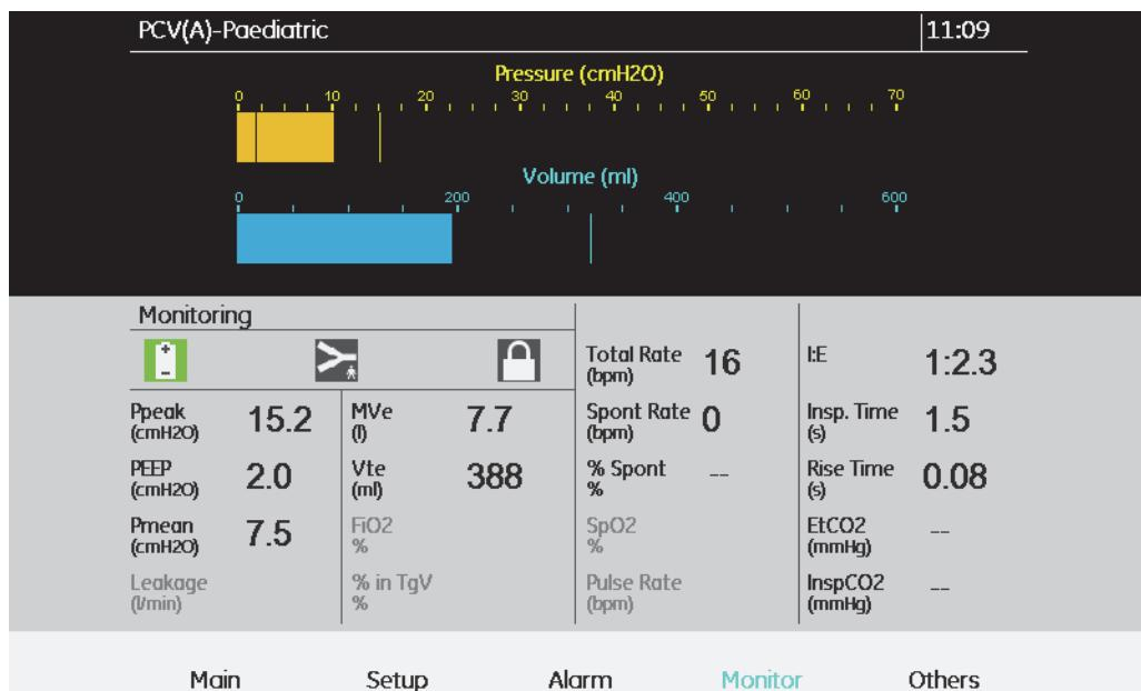
The monitoring screen contains a bargraph field that displays current Pressure, PEEP and  $P_{\text{peak}}$ , pressure and volume alarm limits, and inspired/expired tidal volume. The monitoring field displays all available values for the current treatment mode. (In most other screens, except for the curve and trend view, a small monitoring field is displayed with 8 values.) See “Monitored Values in the Vivo 65” on page 52 for a description on the monitored values.
