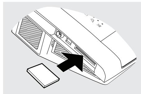
**2** When the memory card is inserted, a pop-up window will appear on the Vivo 65’s display. Press OK to start saving data on the memory card.
