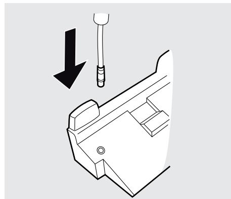
**2** Connect the charger to the AC power supply.
